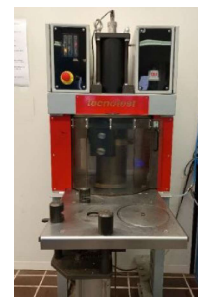
Compaction at fixed height = 180 mm
