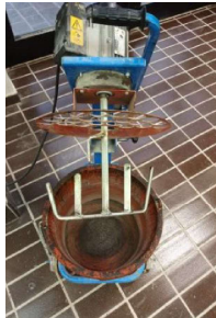
The surface of the mixer bin has been moistened
