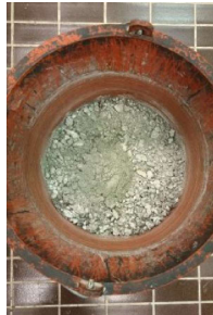
The cement is added (CRM1-63 g, CRM2-126 g)
