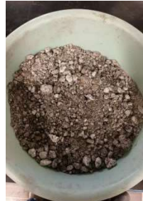
After newly mixing, resulting RA + Filler + W_{abs}
