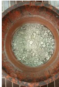
The material is unwrapped and put in the mixer bin
