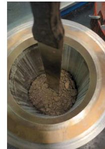
The mixture is slightly compacted with a spatula
