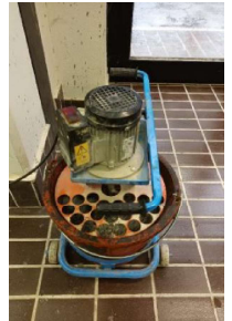
Mixing all the solids – mixer (about 1')
