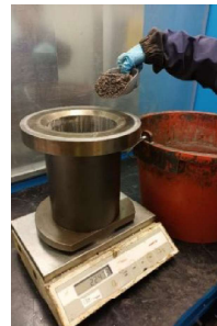
A disk is put at the bottom. The mixture is put in the mould.
