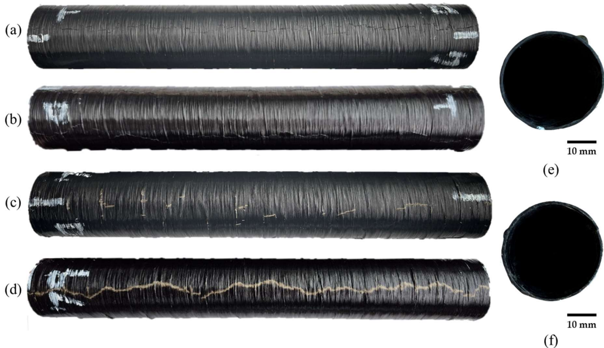
Figure 8. Macroscopic observations of the fracture of specimens subjected to radial compression tests: (a) contact surface with plate, (b) side surface, and (e) cross-section of the CFRP specimen; (c) contact surface with plate, (d) side surface, and (f) cross-section of the BFRP specimen.
