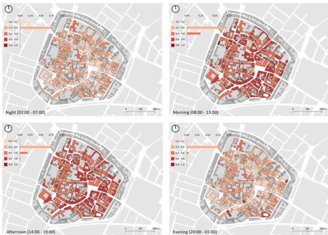
Fig. 11. Maps of UEV over time, classified according to the general ranges adopted in this study, with bar charts showing the proportion of buildings in each class for the different time slots.
