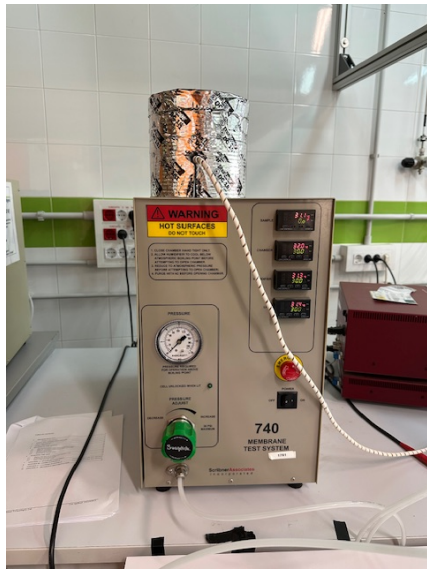
Figure 1: Membrane Testing System for through-plane membranes conductivity measurements.
