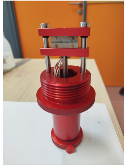
Figure 2: Cell Head for through-plane membranes conductivity measurements.
