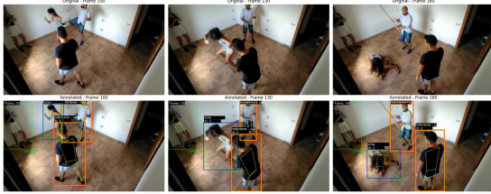
Fig. 3: Comparison between original frames (top) from violent videos and the same frames with keypoints overlaid (bottom).
