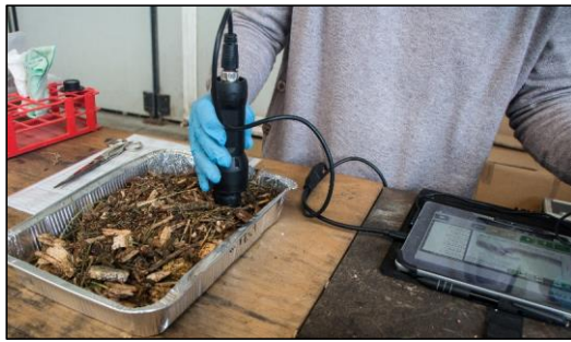
178 Figure 1: portable MicroNIR™ OnSite sensor application on industrial woodchipwood chip pile in power plants (left) 179 and in laboratory (right).
