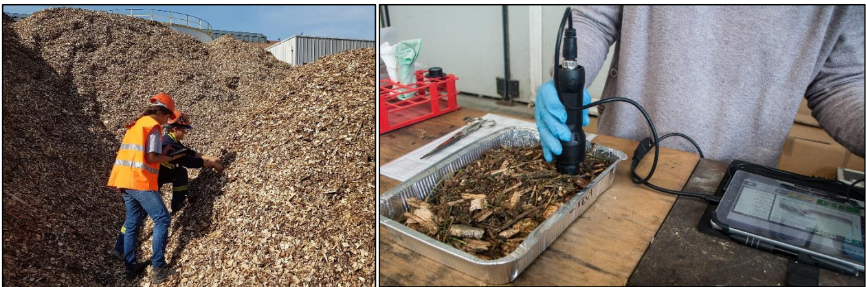
159 Figure 1: portable MicroNIR™ OnSite sensor application on industrial wood chip pile in power plants (left) and in 160 laboratory (right).
