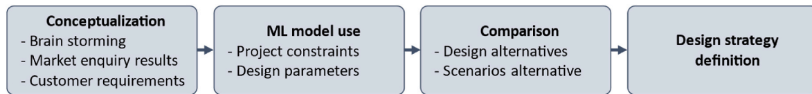
Fig. 6. ML model workflow in EVs concept design.
