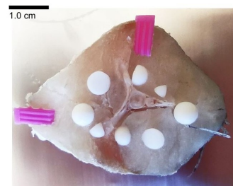
Fig. 2. Experiment 2: Truncated cone-shaped fish sample with eight white plastic inserts, including whole spheres, half spheres, quarter spheres eighth spheres and two pieces of pink HDPE
