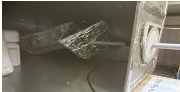
Fig.1. The Reverberation Chamber and its mechanical stirrer.
