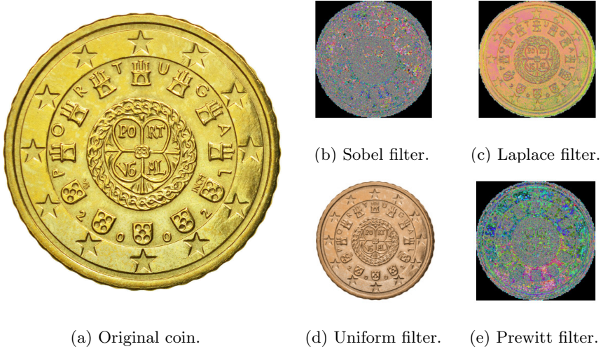
Fig. 5: Example of filters applied on the image of 10 Portuguese cents.
