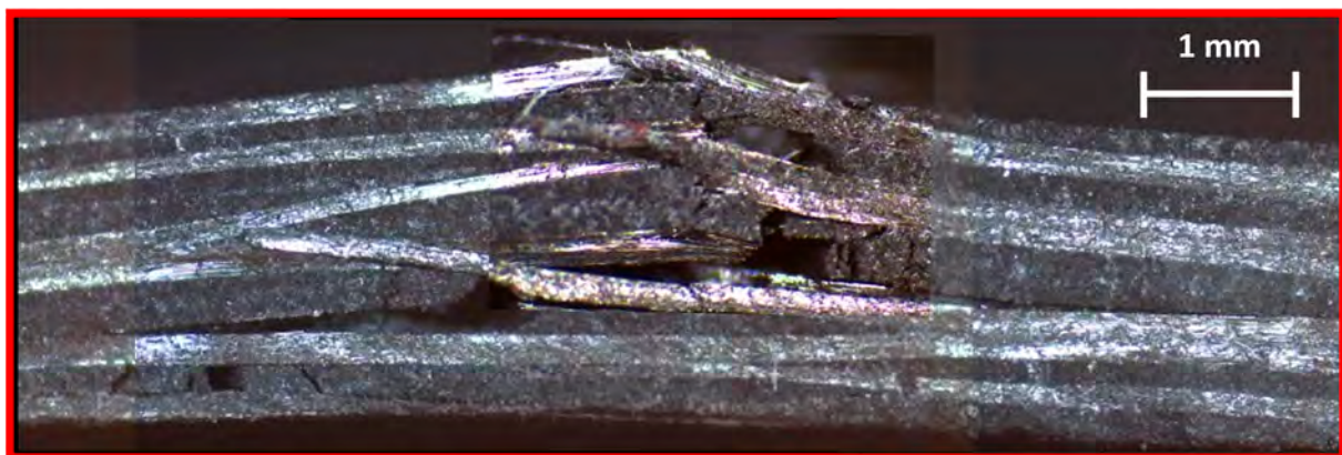
Figure 7. Fractured longitudinal section of a tensile specimen manufactured by laying-up plies of 380 g/m 2 .
