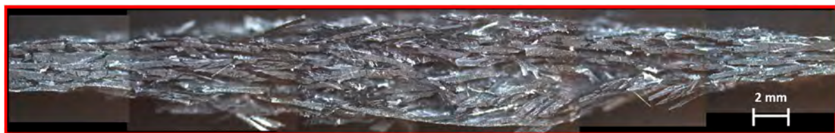
Figure 11. Fractured longitudinal section of the in-shear specimen in composite laminate manufactured by laying-up plies of 630 \text{ g/m}^2 .
