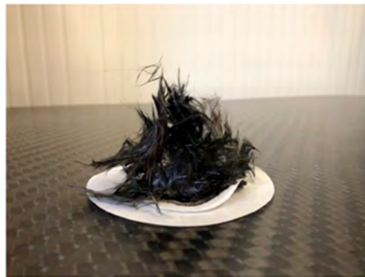
Figure 2. Dry fibers after resin digestion the void quantity analysis.
