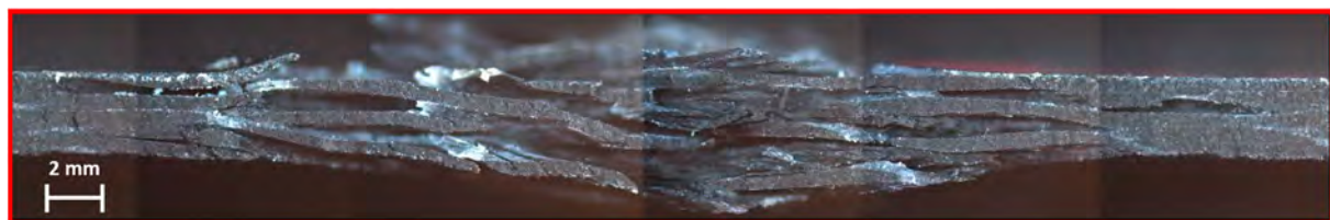
Figure 12. Fractured longitudinal section of the in-shear specimen in composite laminate manufactured by laying-up plies of 800 \text{ g/m}^2 .
