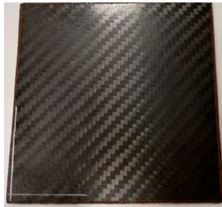
Figure 1. A flat laminate in CFRP produced by hand lay-up process, after curing.
