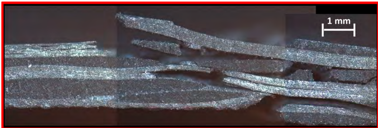
Figure 9. Fractured longitudinal section of the tensile specimen manufactured by laying-up plies of 800 g/m 2 .
