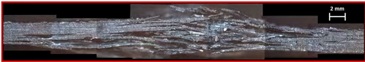
Figure 10. Fractured longitudinal section of the in-shear specimen in composite laminate manufactured by laying-up plies of 380 \text{ g/m}^2 .
