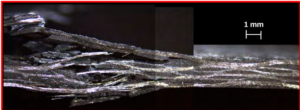
Figure 8. Fractured longitudinal section of a tensile specimen manufactured by laying-up plies of 630 g/m 2 .
