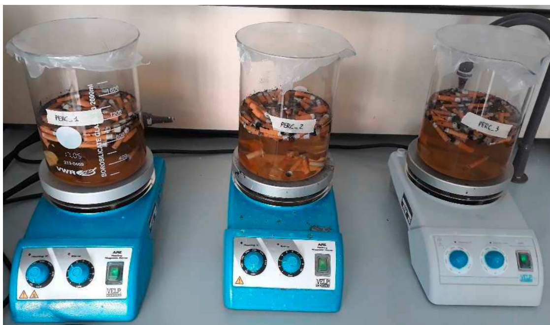
Figure 3.1. Cigarette butt leachates preparation: CBs soaked in ASW for 24 hours in agitation on a magnetic stirrer. These leachates are referred to the triplicates of LEAC_A (100 CBs/L) = PERC_1, 2 and 3.
