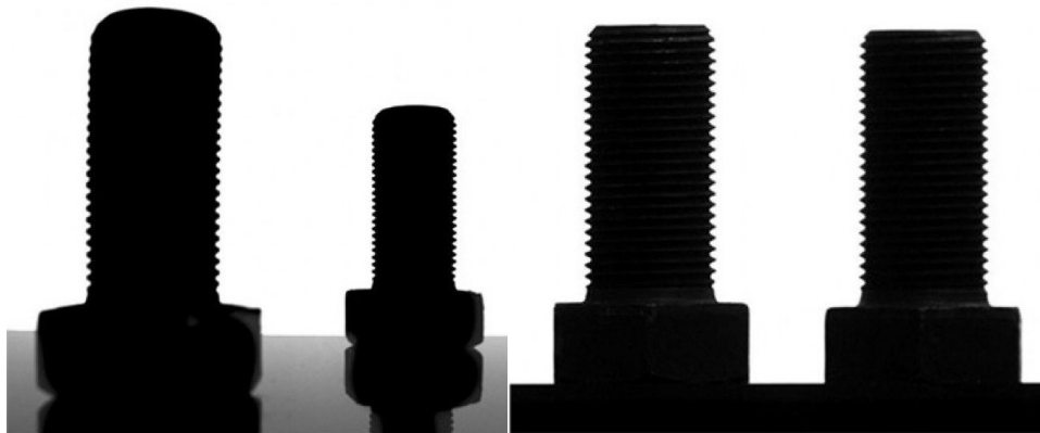
Figure 38. (Left) Proportional effect of standard lenses: two identical screws, placed at different distances appear as having different sizes. (Right) Telecentric view: the same two screws, placed at different distances, appear identical.
