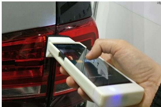
Figure 100. Phone case integrating the laser-line triangulation system [80].
