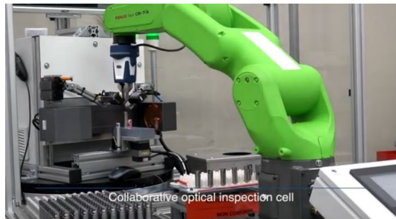
Figure 6. Collaborative optical inspection cell, photo by Z4tec. Example of robotic arm performing pick and place measurements [31].
