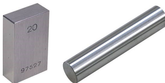
Figure 67. Gauge block of 20 mm (Left) and pin of 12 mm (Right) used as reference measurands.
