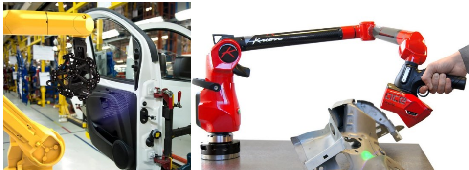
Figure 7. (Left) Example of a robotic arm holding a sensor for quality inspections. Photo by Creaform [32]; (Right) Photo of Ace arm by Kreon [33].
