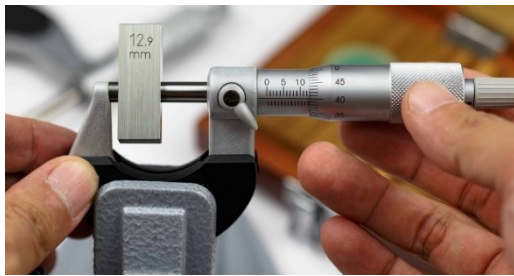
Figure 29. Manual micrometer. Photo by [82].
