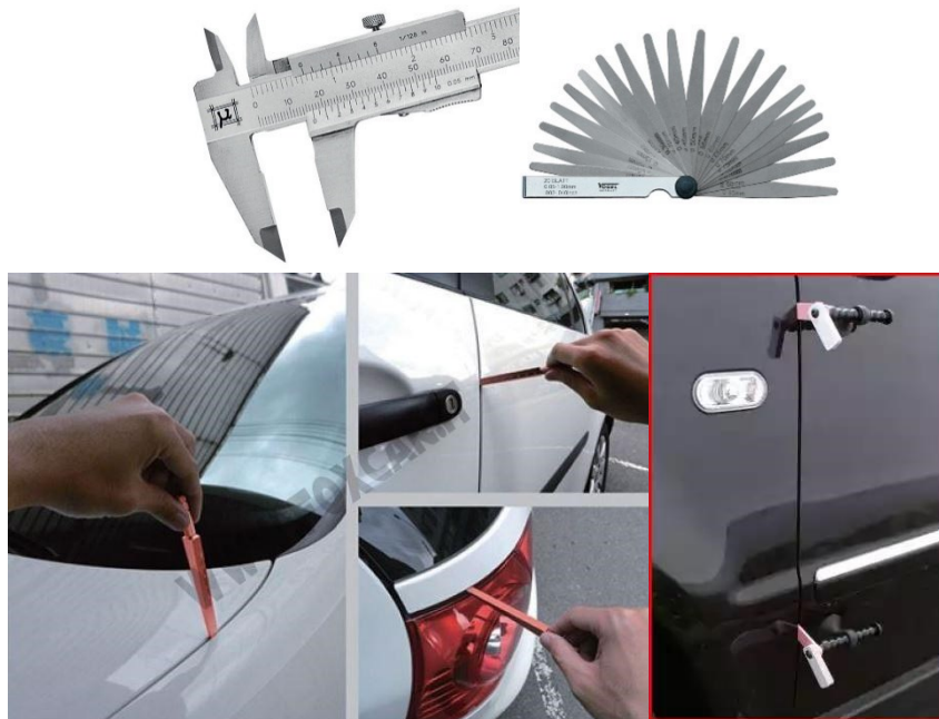
Figure 19. Examples of manual measurements of gap and flush: (Top) a caliper [56] and feeler gauge [57]. (Bottom) feeler gauges used on car body [58] [59].
