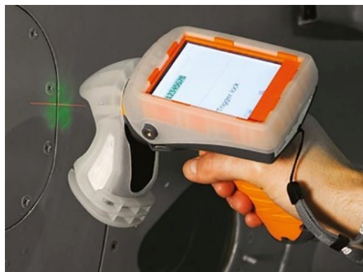
Figure 26. GapGun Pro 2 by QFP [77].
