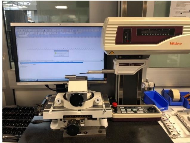
Figure 45. Laboratory surface roughness tester by Mitutoyo.
