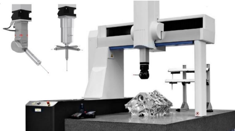
Figure 32. Coordinate Measuring Machine with different types of probes. Photo by [84].
