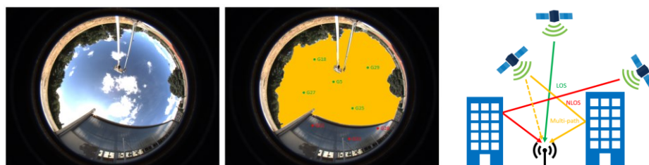
Figure 20 Left side: sky representation with projected satellites (green = LOS; red = NLOS). Right side: schemes of the multipath and NLOS effect. (Feriol et al. 2020)
