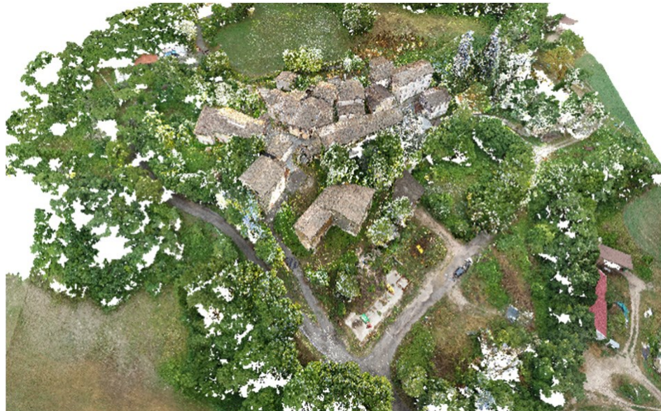
Figure 5 Unified lidar and photogrammetric point cloud
