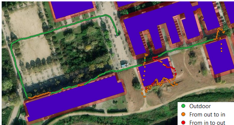
Figure 35 MK test applied to the trajectory of CTTC campus. Green points are good GNSS areas, orange are transitional areas from outdoor to indoor and red are from indoor to outdoor
