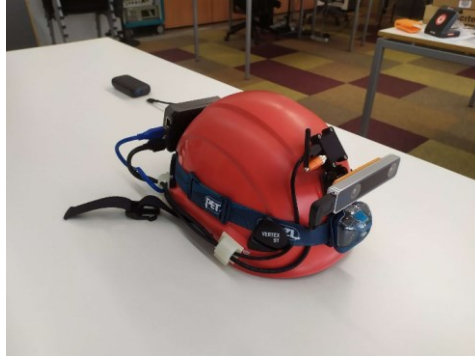
Figure 18 Positioning system mounted on a helmet designed and built by CTTC
