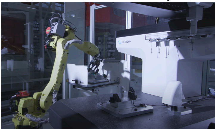
(b) Hexagon 3D coordinate measuring machine
