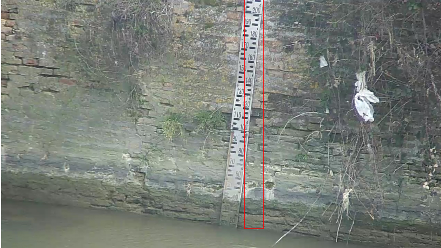
Figure 5.24: The original frame with the desired gauge positioning, used to compute image rectification settings.
