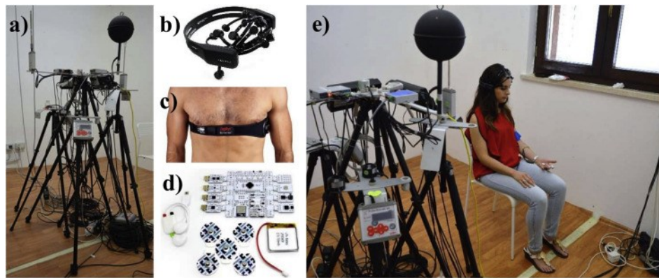
Figure 10. Experimental set-up: (a) microclimatic station, (b) EEG sensor EPOC+, (c) Zephyr Bioharness 3.0, (d) BiTalino sensor, (e) representation of the participant during the experiment.
