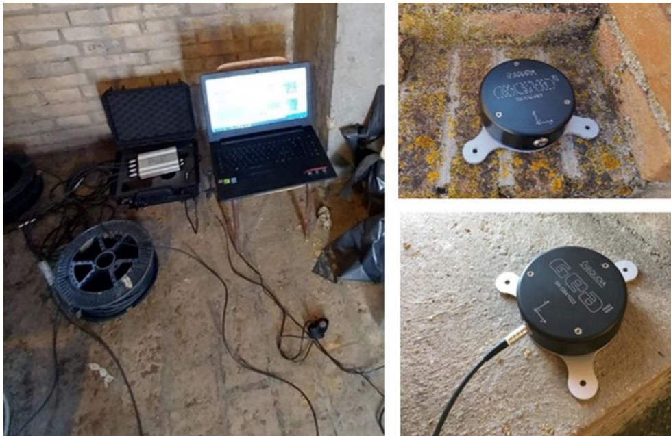
Figure 13: Instrumentation used for the ambient vibration tests.
