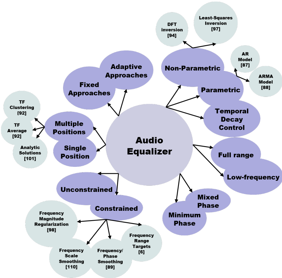
Figure 4.1: Diagram of Multipoint Audio Equalization aspects.
