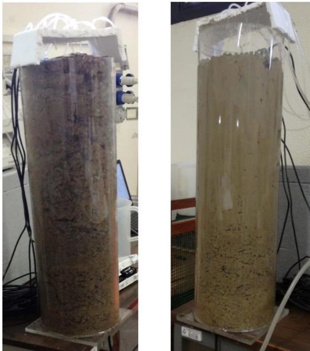
557 Figure 10: Soil column at initial (left picture) and final (right picture) conditions, after the clay's 558 swelling due to the compost addition in the topsoil.
