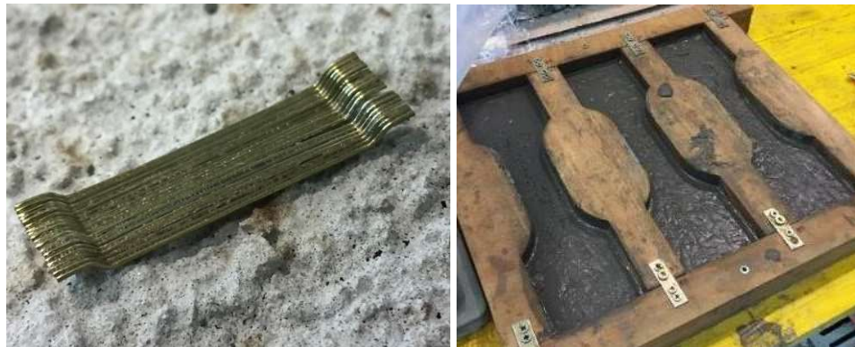
Figure 1. Hooked steel fibers and dog-bone shaped specimens manufacturing.
