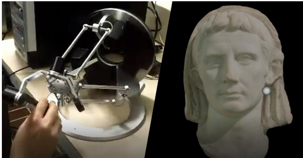
Figure 2: The proposed haptic interface, based on the Omega 6 produced by Force Dimension.
