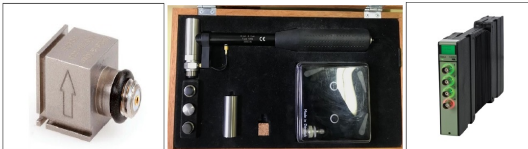
[2] 1. Beam 2. Accelerometer 3. Impact hammer 4. Analyzer FFT
