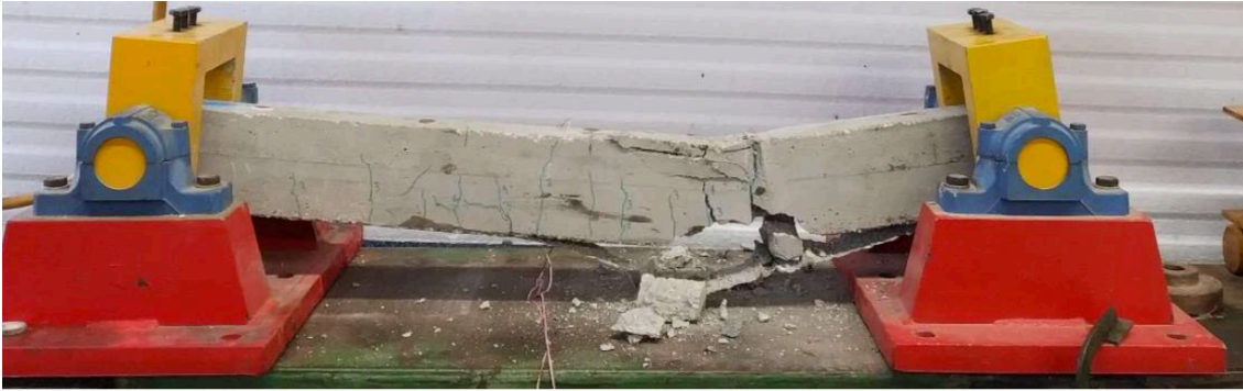
Figure 20 – View of failure of strengthened beam type B with detail of GFRP rupture.
