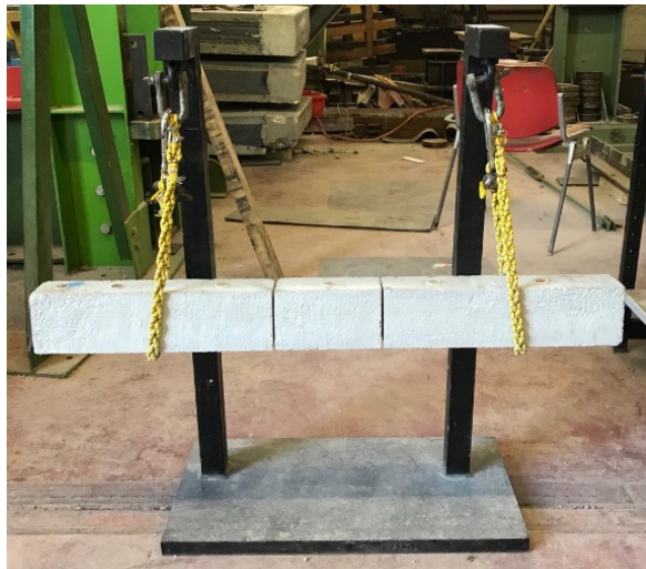
Figure 12 – Set up for vibration tests of beam type C with symmetric damage by notches.
