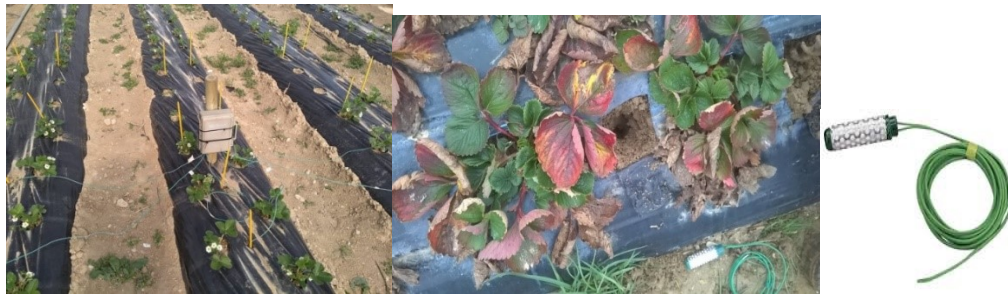
Figures 12-13: Record-keeping system of tensiometers and the measurement site with tensiometer probe
